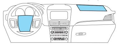
The airbag supplemental restraint system (SRS) is designed to work in conjunction with the safety belts to help protect the driver and front outboard passenger from certain upper body injuries. The term "supplemental restraint" means the airbags are intended as a supplement to the safety belts. Airbags offer the most protection when used with safety belts for crash conditions for which airbags are designed to deploy. Airbags do not offer any protection in crashes for which they do not deploy.
